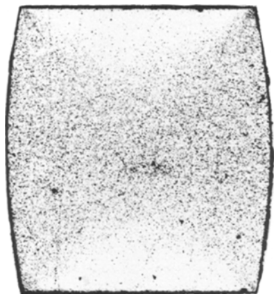
Figure 2 Longitudinal section of MgO specimen after 16% creep strain at 96 \text{ MN m}^{-2} and 1596 \text{ K} , \times 10 .
